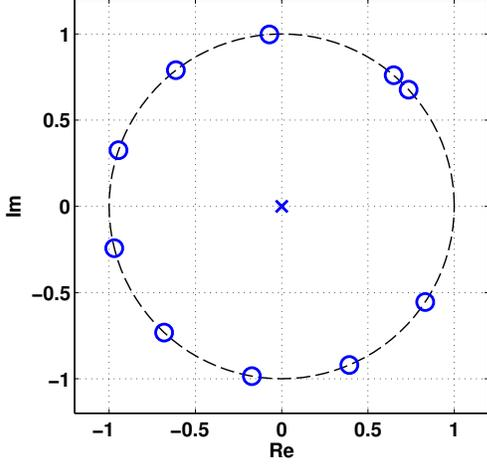
**Fig. 1.** Zero locations of MVDR beamformer using  $N = 11$  element ULA.
