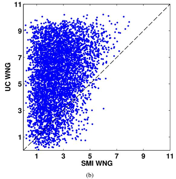
**Fig. 5.** Comparison between WNG for UC MVDR and SMI MVDR beamformer with  $N = 11$  element ULA and  $L = 12$  snapshots.
