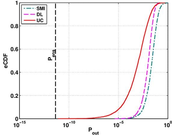
**Fig. 4.** Comparison of interferer output power empirical CDF between UC MVDR, SMI MVDR and DL MVDR beamformers with  $N = 11$  element ULA and  $L = 12$  snapshots.
