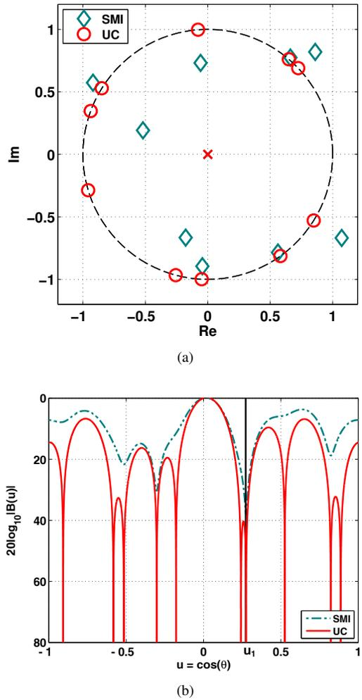
**Fig. 3.** Zero locations and beampattern for representative example of SMI MVDR and UC MVDR beamformer using  $N = 11$  element ULA for  $L = 11$  snapshots.
